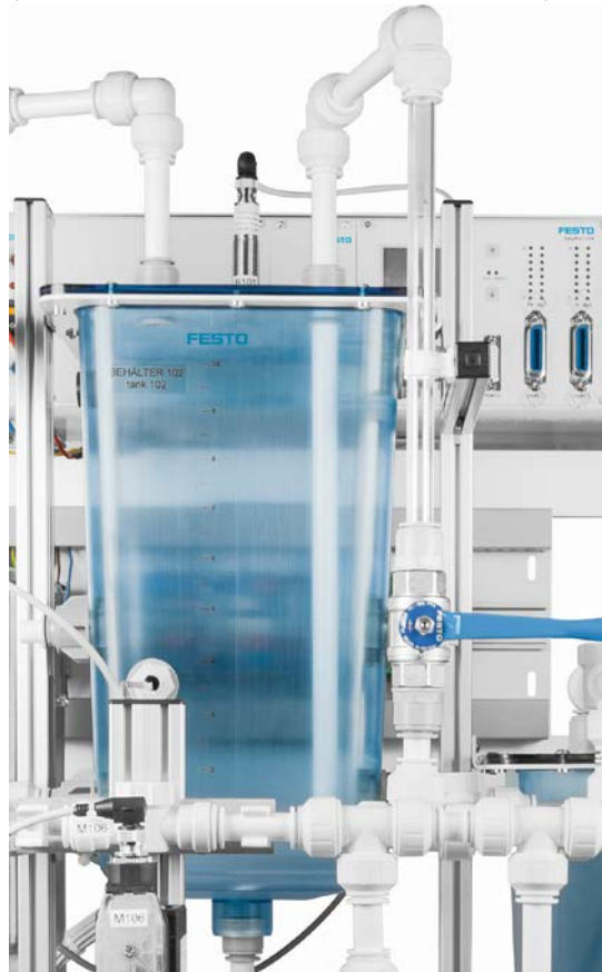
Controlled level system – ultrasonic sensor B101 (measuring point 'LIC BL1') for basic design
